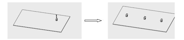
3. Drill 8-12mm outlet holes on the installation surface of the input end of the strip, and pull out the wire and connect it with the input wire of the strip.
